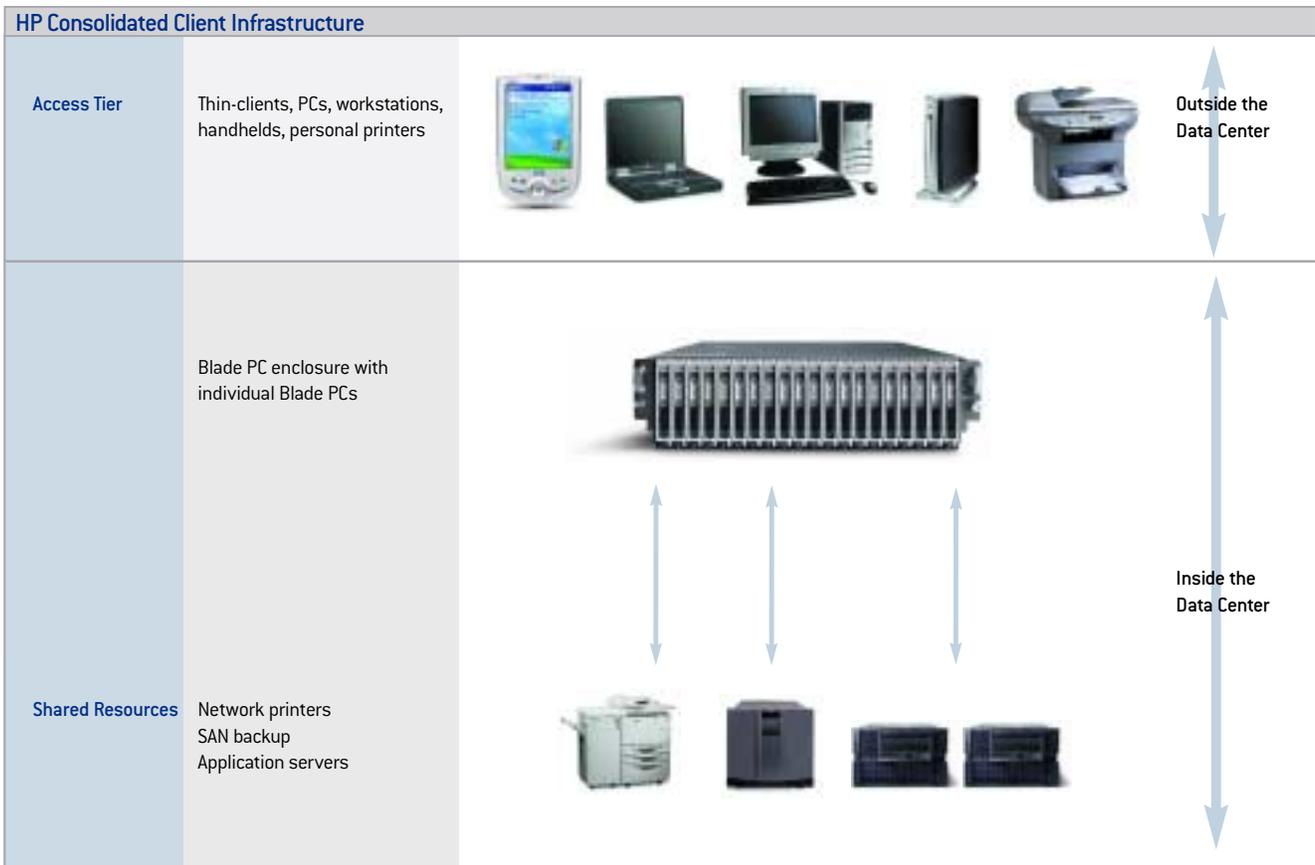
HP’s Consolidated Client Infrastructure (CCI) solution is a blade PC strategy that establishes a one-to-one connection between end-users and dynamically allocated blades and centralized storage. Desktop images and data are stored and controlled in the data center. End-users access their desktop images from any device — thin-clients, tablets, PCs, workstations and handhelds — anytime, anywhere.
